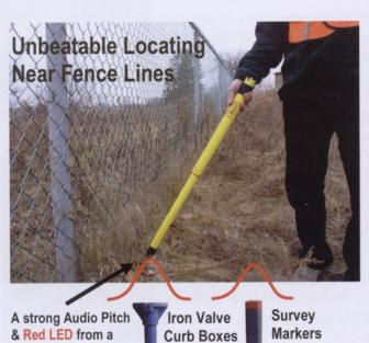
Hold the locator at an angle to the Fence the **Mode Tone** and **Green LED** will then appear. Next move the locator along the fence line. When a **Strong Audio tone pitch** & **Red LED** appears this will indicate a possible vertical target.
